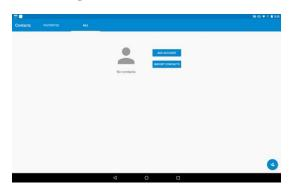
The first time, please choose to import contacts, support various ways to add contacts. You can import SIM card, SD card contacts, or set up the synchronization account, you can also create a new contact directly
