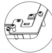
Step 4: Tighten the M4x8mm & M2.6x8mm screws to secure the bracket and tighten the longer M4x20mm screws to secure the monitor againstst the panel.
