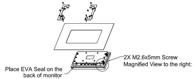
Remove 2X M2.6x5mm screws before installing bracket
