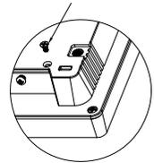
Step 1: Create panel cut out, remove two M2.6x5mm screws and place EVA seal
