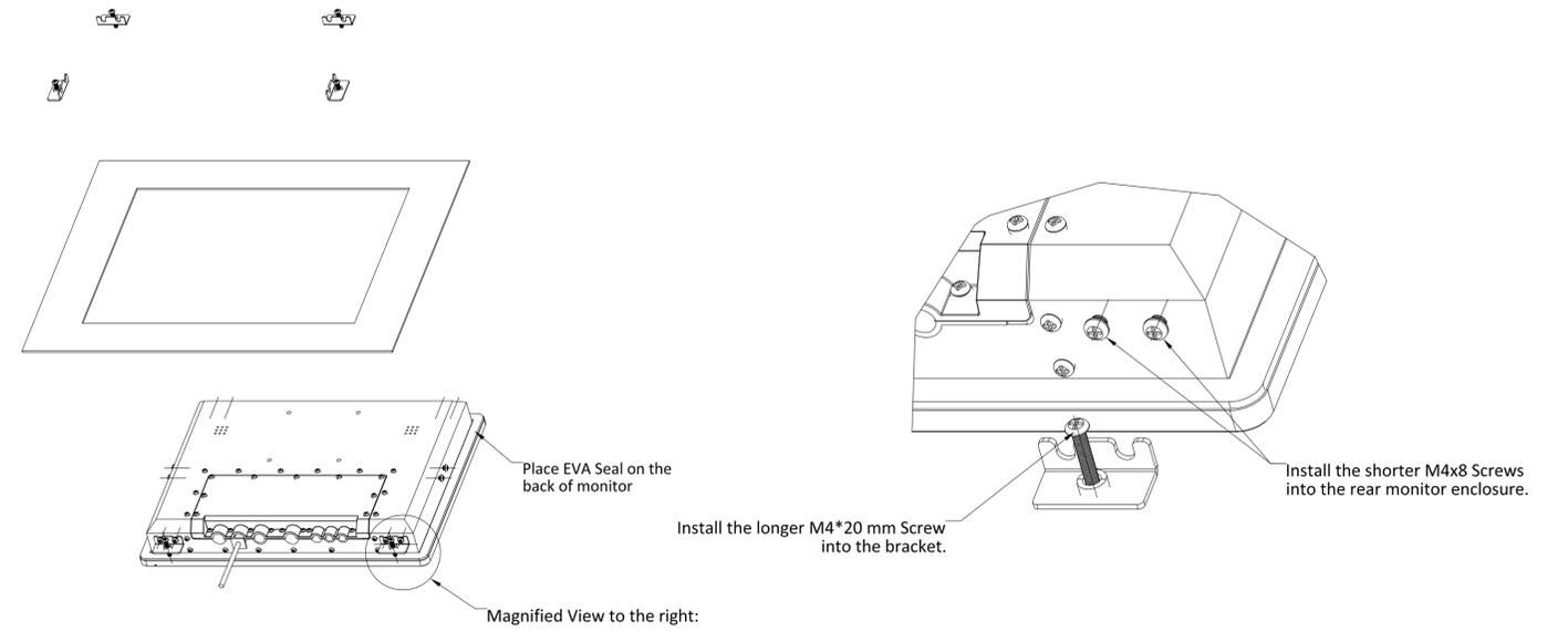
Step 1: Create panel cut out, place EVA seal, and install two bottom brackets.
