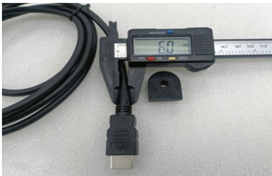
P3. Diameter of HDMI cable: 6mm.
