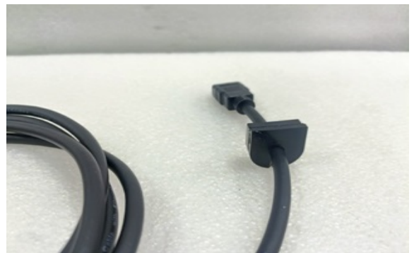
P4. Install Rubber Grommet onto HDMI cable.
