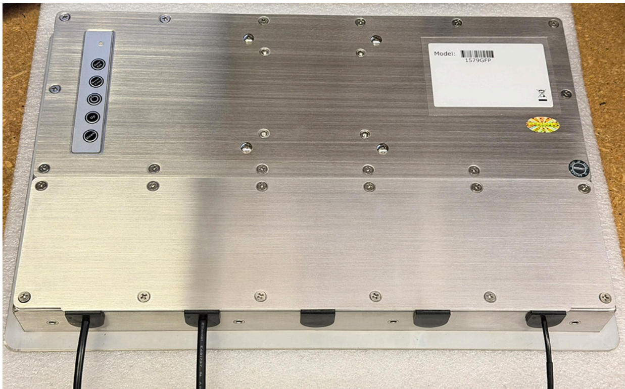
P6. Please ensure that the Rubber Grommets are pushed to the very bottom in order to guarantee the best water protection.
