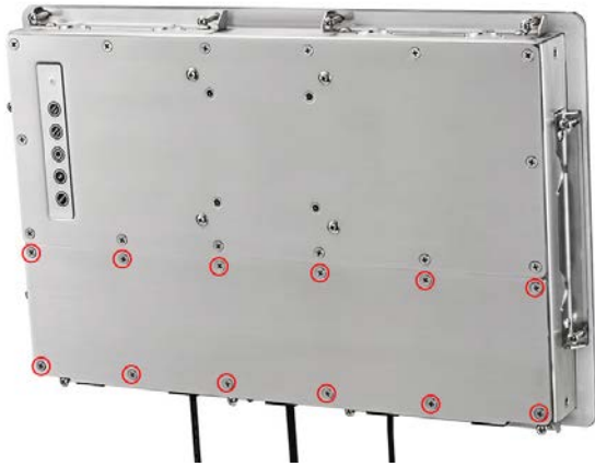
P1. Remove 12 Screws holding the cover
